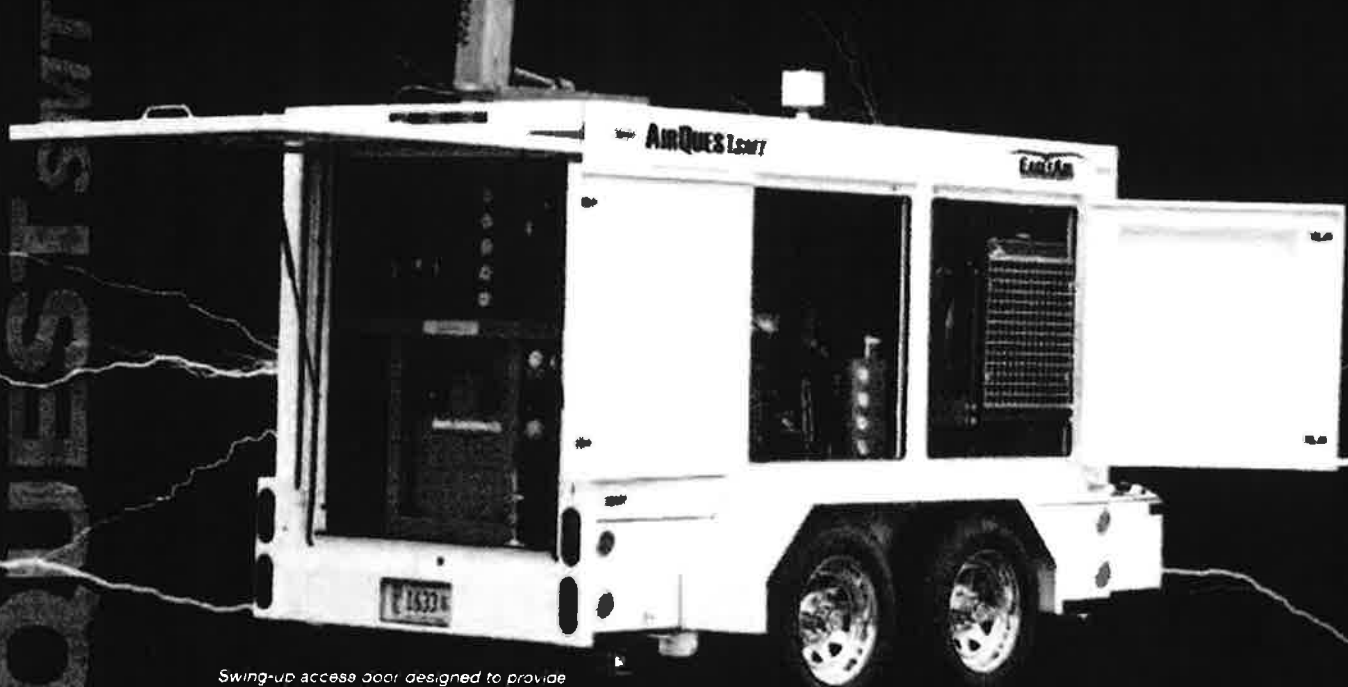
Swing-up access door designed to provide operator shelter from the elements
