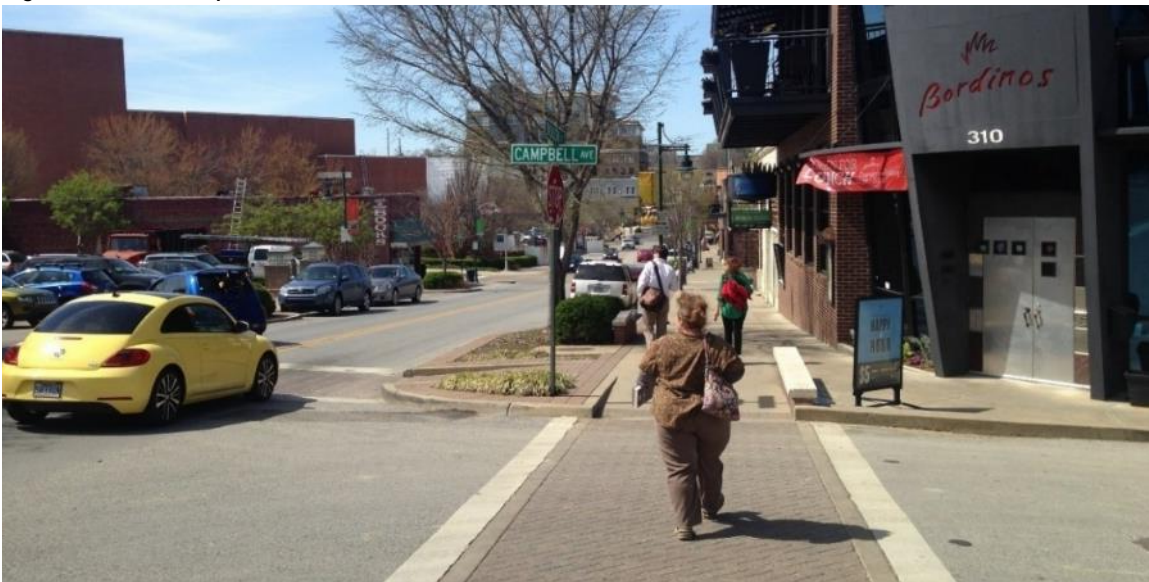
Figure 28 Example of Textured Crosswalk - Dickson Street
