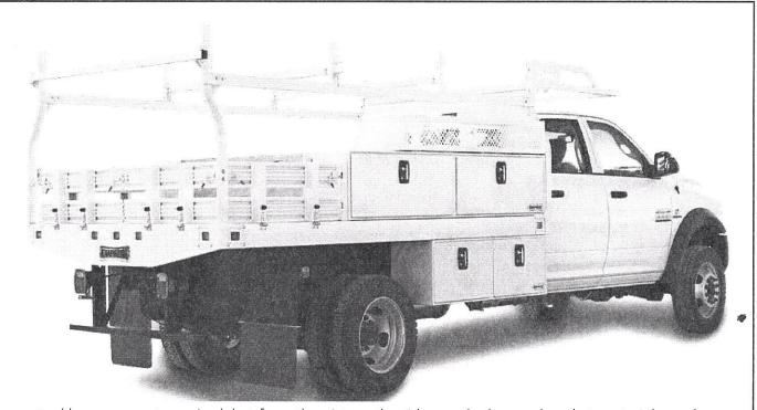
The upper tool boxes are not required, but from the picture the sides can be lowered so that materials can be loaded.
