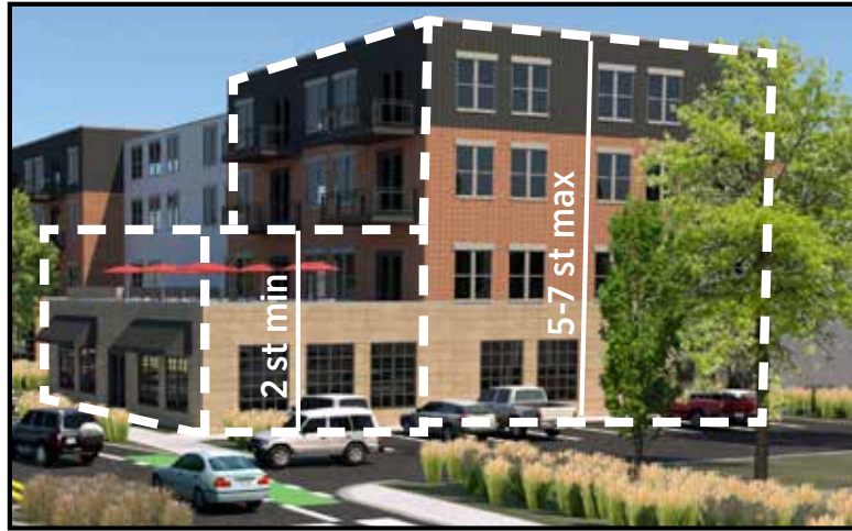
Step-back building concept at Urban Place nodes. The possible regulation permits a two (rather than three)-story minimum height at the building line, provided that the project includes a higher building, consistent with UT requirements, behind.
